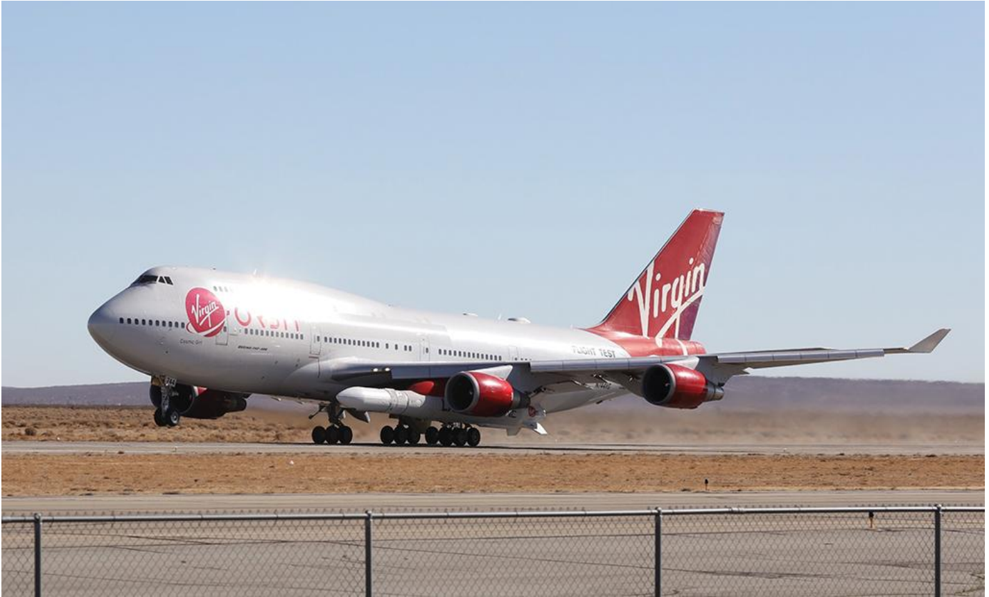
A Virgin Orbit Boeing 747-400 carrier aircraft lifts off from Mojave Air and Space Port with the 57,000-lb. LauncherOne attached under its left wing. Credit: Virgin Orbit
