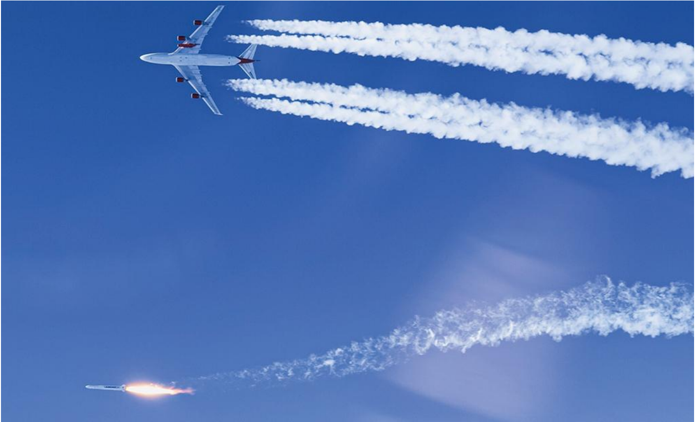
LauncherOne's Newton 3 engine started just over 5 sec. after release from the Boeing 747-400. Credit: Greg Robinson/Virgin Orbit
